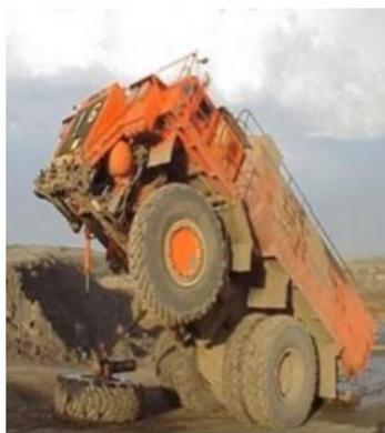
Gambar 36. Ban *Water tank truck* terlepas
