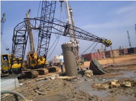
Gambar 55. Jib *Crawler crane* Patah
