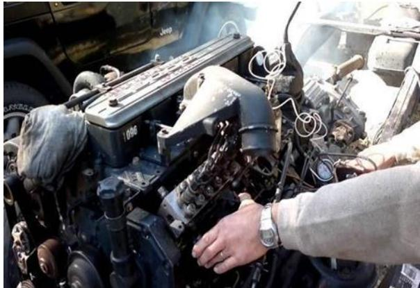
Gambar 56. Mesin *Crawler crane* Overload
